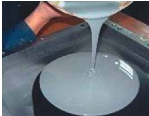
Fig. 8 – Resin deposition on the master
