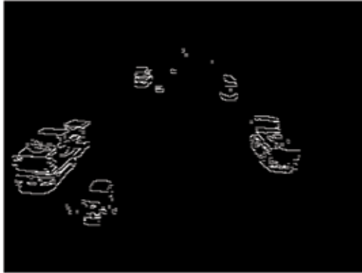
Figure 4: Edges detected by applying the Canny Edge Detector to the Background image.
