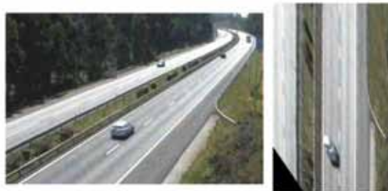
Figure 13: Example of a captured image (on the left) and the correspondent rectified image (on the right).
