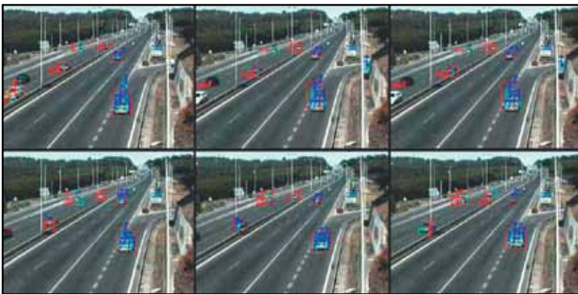
Fig. 7. Wrong way drivers detection in real event video sequence. All the moving vehicles were validated as wrong way drivers.
