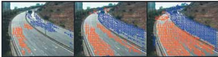
Fig. 3. Three frames showing the evolution of the orientation pattern modeled by the first Gaussian of the GMM on a highway scenario.
