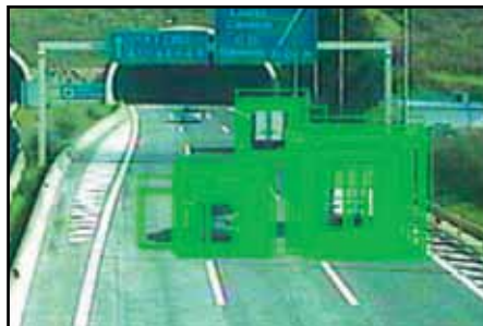
Fig. 6. Cars classification using AdaBoost classifier at different scales and positions of the search window on the image.
