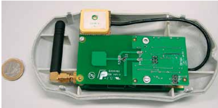
On Board Unit Interoperability (OBUi) DSRC/GNSS device prototype
