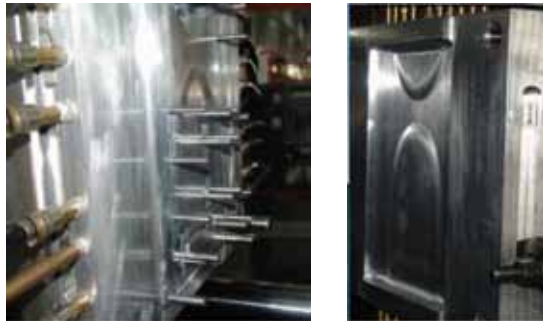
FIG. 4. – Core and cavity of aluminium mould
