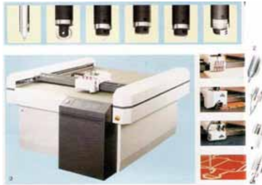
Fig. 6 – Example of CNC machine (and tools) for paper cutting and stressing [7]
