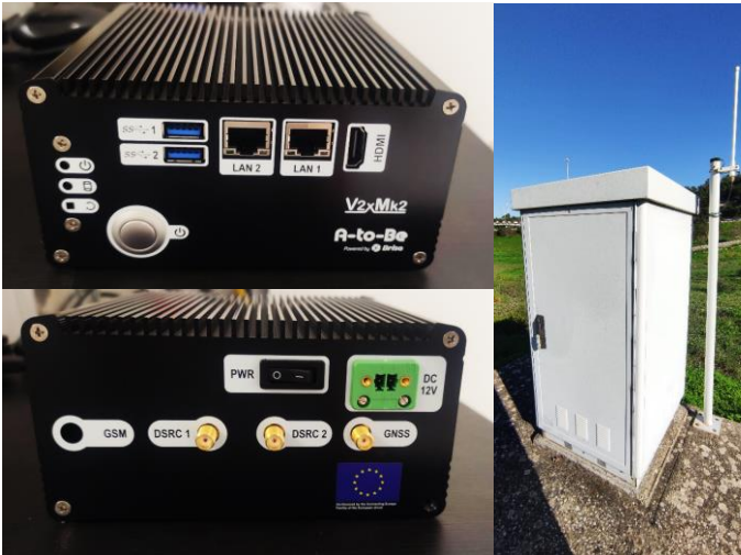
Figure 2 – Roadside Equipment (ITS-G5 unit on the left and enclosing cabinet on the right).
