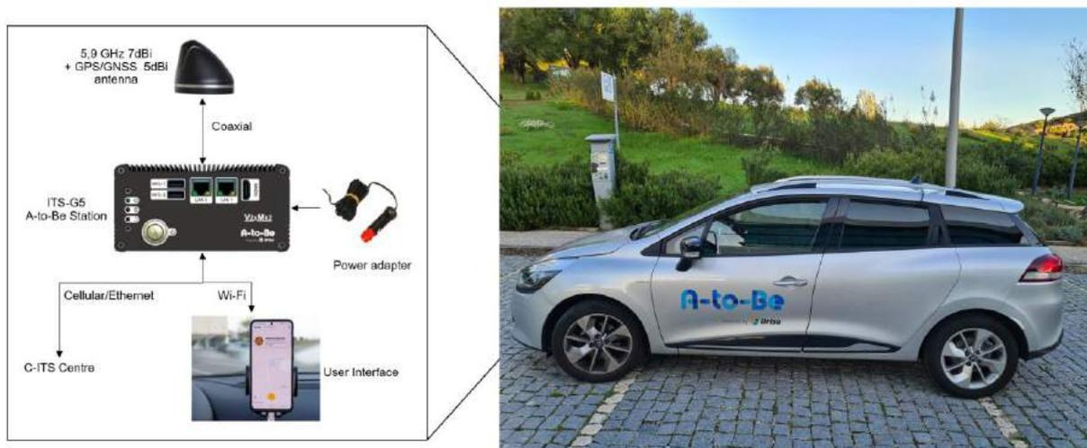
Figure 5 – A-to-Be V-ITS-S solution
