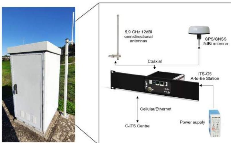
Figure 4 – A-to-Be’s R-ITS-S solution
