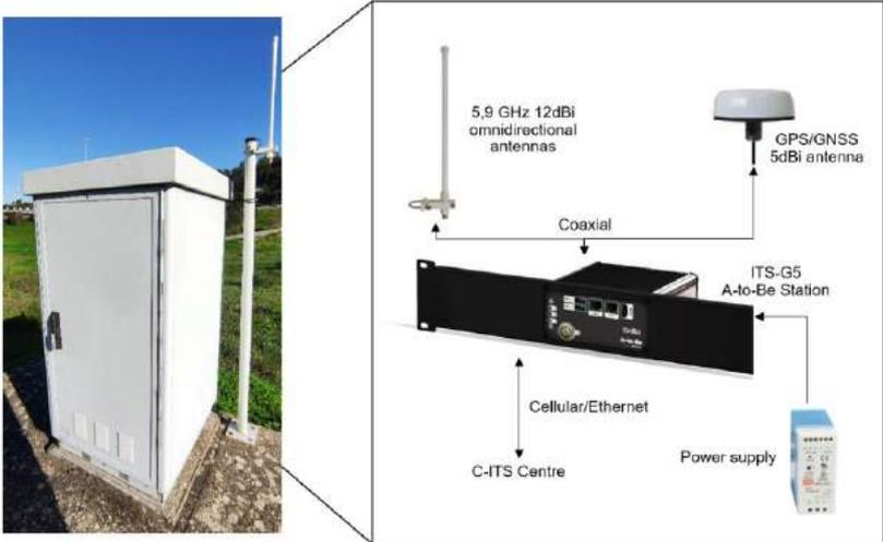
Figure 4 – A-to-Be’s R-ITS-S solution
